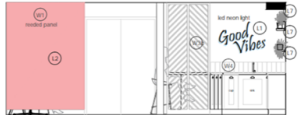
B 4 ELEVATIONS | END OF BREAKFAST BAR | OPTION TWO - BLACK TIMBER SCREEN SCALE 1:20
