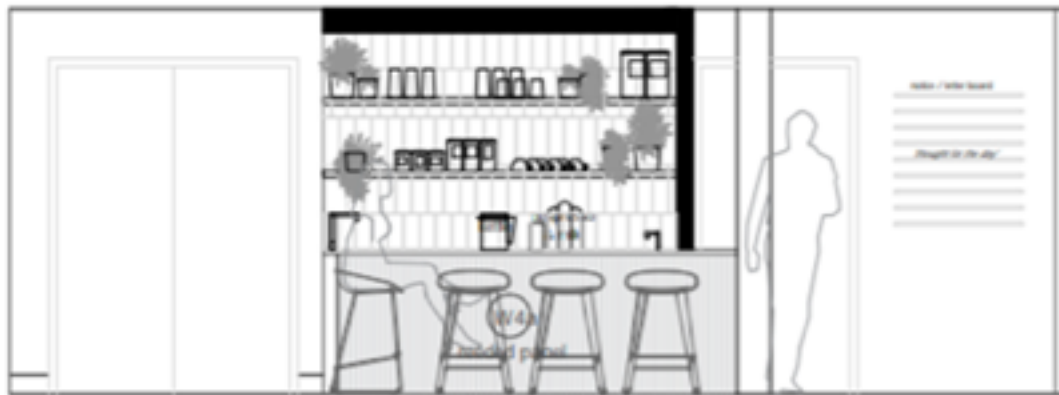
A 3 ELEVATION | FRONT FACE OF TEA PREP / BREAKFAST BAR SCALE 1:20
